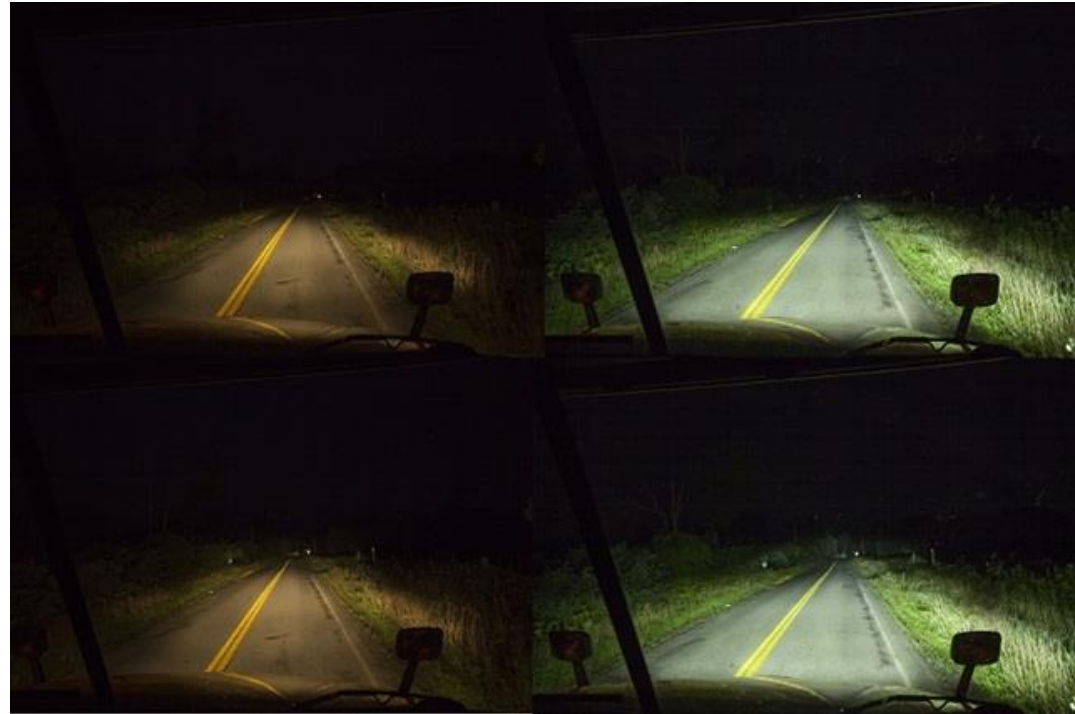
Comparison between Halogen and LEDs lights with high and low beam ( www.truckinginfo.com )
