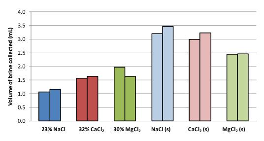
Figure 12: Modified SHRP Ice Melting Test results at 60 minutes at 15°F
