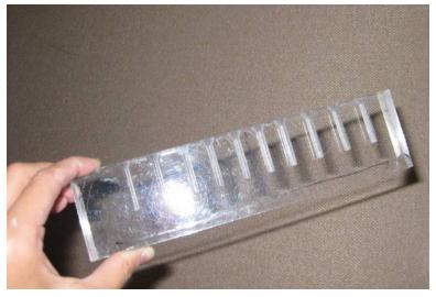
Figure 13: SHRP Ice Penetration Test apparatus
