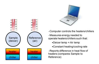
Figure 5: Concept of Differential Scanning Calorimetry (DSC)
