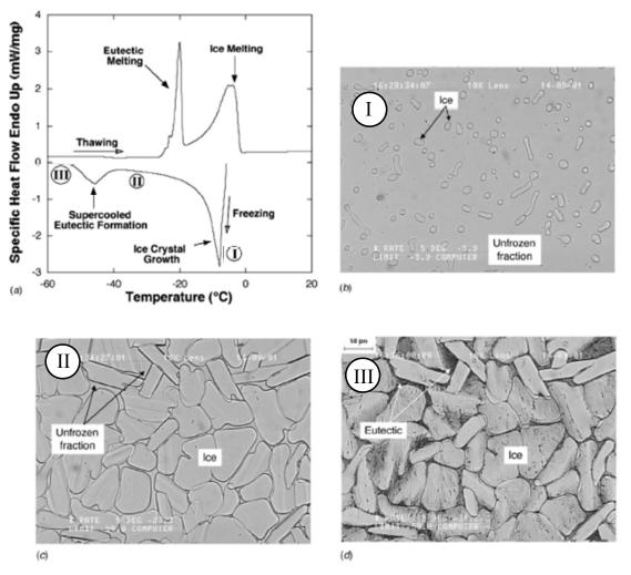
Figure 7: DSC thermogram and cryomicroscopy images during freezing/thawing of a simulated salt brine (adapted from Han and Bischof, 2004)
