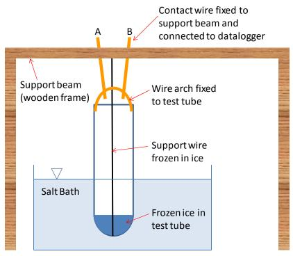
Figure 15. Mauritis Ice Undercutting Apparatus
