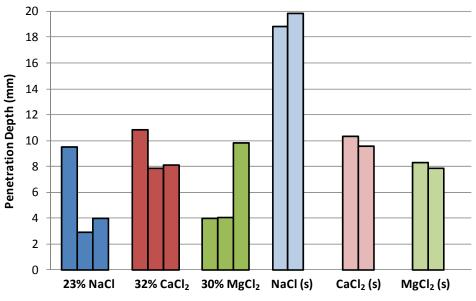
Figure 14: Modified SHRP Ice Penetration Test results at 60 minutes at 30°F
