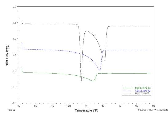
Figure 8: DSC thermograms of 23% NaCl, 32% CaCl<sub>2</sub>, and 30% MgCl<sub>2</sub>, dilution 3:1, warming cycle, 3.6°F/minute
