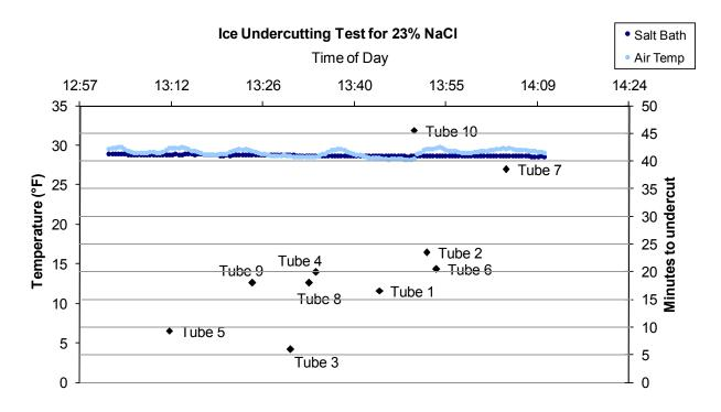
Figure 16: Sample result for ice undercutting test using 23% NaCl at 30°F
