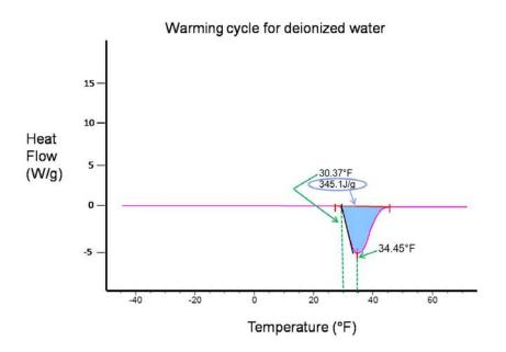
Figure 6: DSC thermogram of deionized water, warming cycle, 3.6°F/minute.
