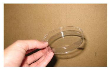
Figure 10: Petri dish used in Modified SHRP Ice Melting Test
