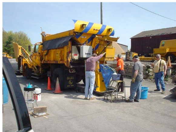
Figure 4-3 Spreader truck's rear wheels raised off ground with hydraulic jacks.
