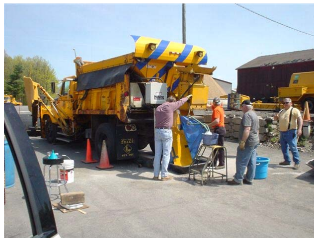
Figure 3-1 Example of having the truck jacked up to conduct drop tests in New York.
