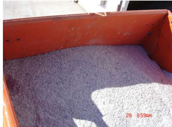
Figure 5-4 Photo showing tailgate auger fully charged during the calibration process.
