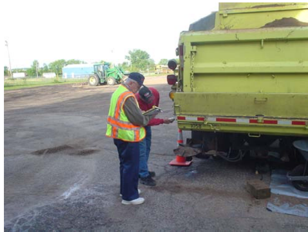
Figure 6-10 Measurement of revolutions of an auger/conveyor shaft for various control settings using a hand-held tachometer.
