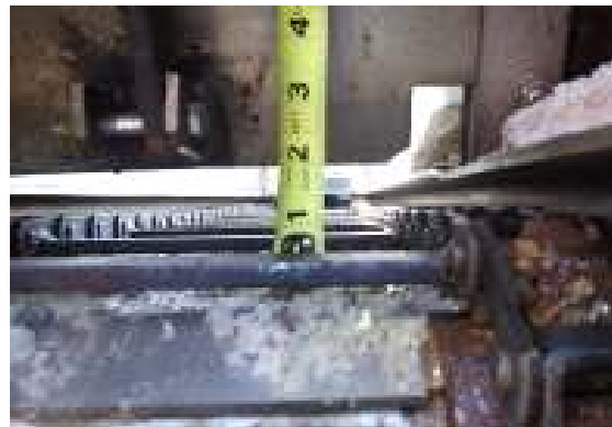
Figure 5-2 Selection of an appropriate single gate opening for range of application rates to be used.
