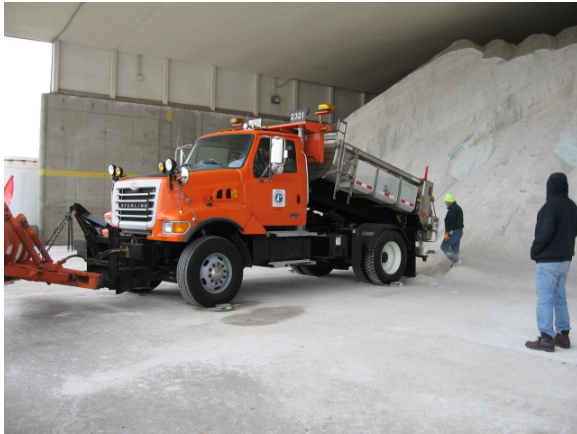
Figure 6-3 Truck-bed raised to an operational elevation for calibration.
