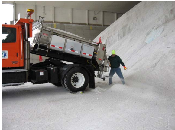
Figure 4-14 Large discharged weights of dry solid material dumped directly on to the solid storage pile.
