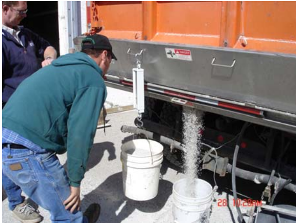
Figure 4-12 Dairy scale used to weigh a 5-gallon plastic bucket with solid discharged material.
