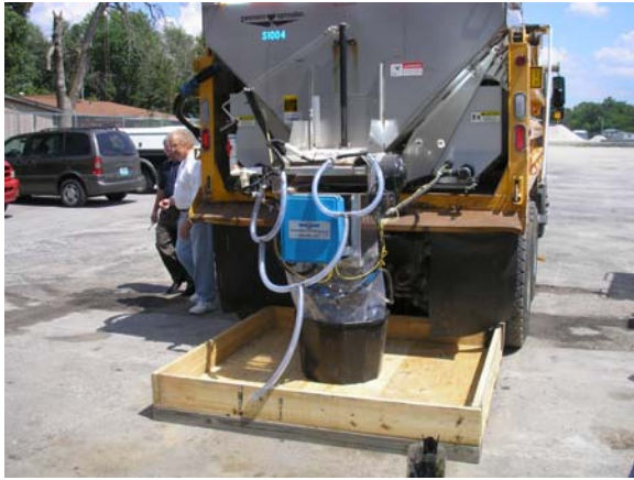
Figure 4-8 Single containment box used to collect up to 200 lbs of discharged dry solid material.
