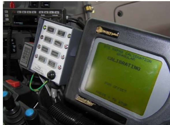
Figure 5-8 Photo of controller display showing unit is in calibration mode.
