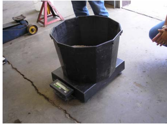
Figure 4-9 Portable scale used to weigh about 100 lbs of discharged dry solid material.
