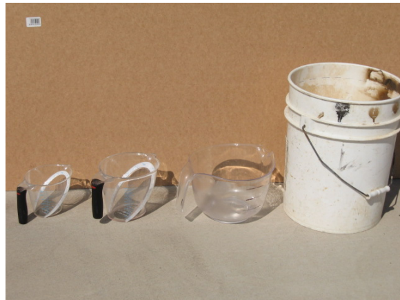
Figure 4-18 Containers for measuring the volume of liquid discharged during calibration.
