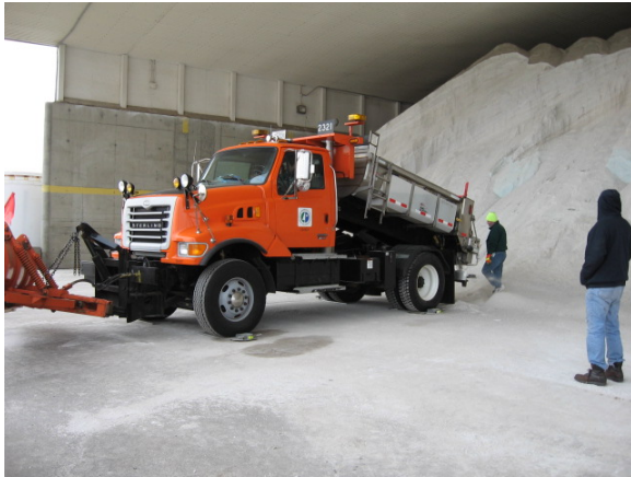
Figure 5-3 Truck-bed raised to an operational elevation for calibration.
