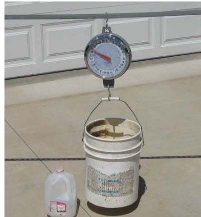
Figure 4-13 A 5-gallon bucket containing three gallons of water suspended from a dairy scale.
