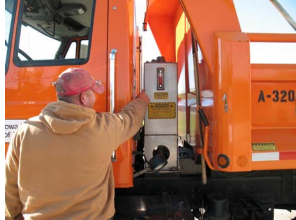
Figure 6-7 Check the operational temperature of the truck's hydraulic oil.
