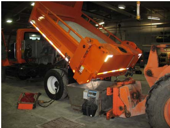
Figure 4-6 IDOT design and built large hopper and load cell used in calibration work.
