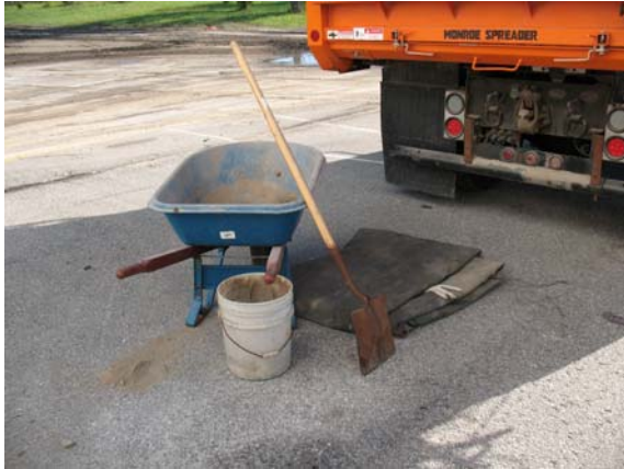
Figure 4-15 Tarp with shovel, broom, and wheelbarrow for collecting solid discharged material.
