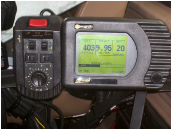
Figure 5-6 Speed readout of 20 mph on the controller in the truck cab.
