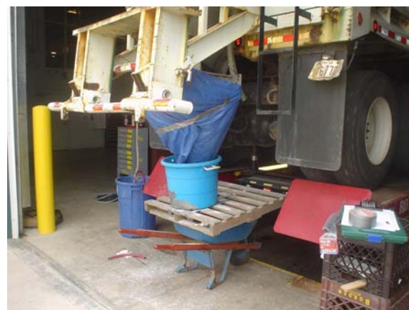
Figure 6-9 Example of conducting drop test with an open-loop controller in Ohio.
