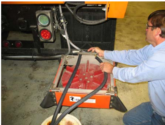
Figure 4-17 Adaptor hose that fits over the spray nozzle to capture the entire liquid chemical discharged during calibration.
