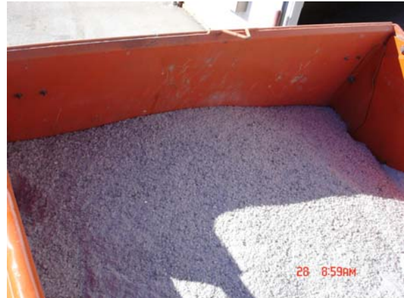
Figure 6-4 Photo showing tailgate auger fully charged during the calibration process.
