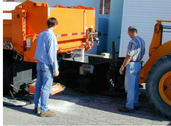
Figure 5-10 Example of using a large hopper with associated weight scale to catch solid material during drop tests in Iowa.
