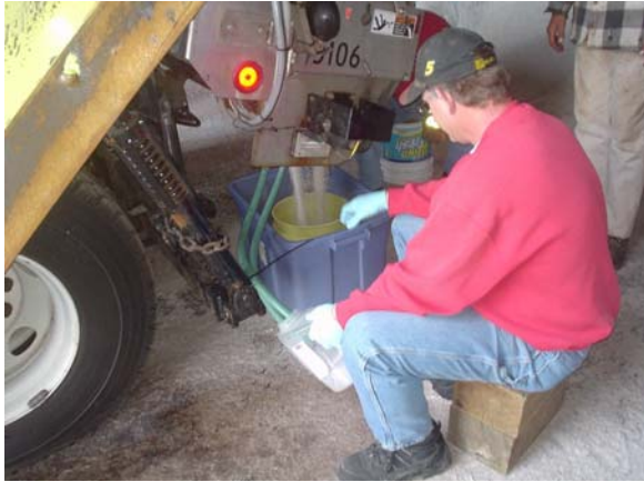
Figure 5-9 Example of solid and liquid materials being collected during drop tests in Wisconsin.
