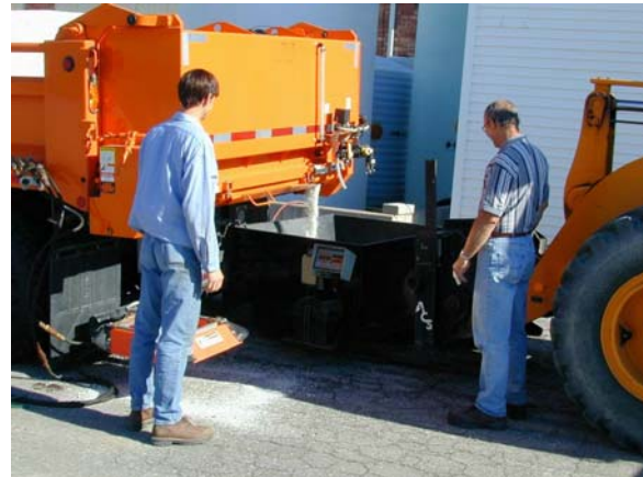
Figure 4-7 IDOT's large hopper and load cell used in calibration work.
