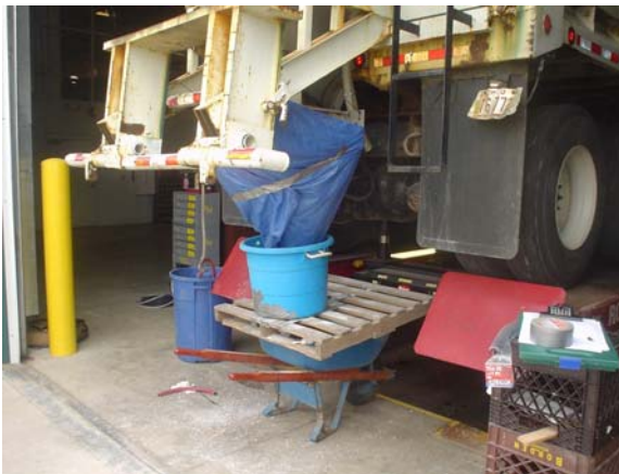
Figure 4-2 Spreader truck on a hydraulic lift for drop tests.
