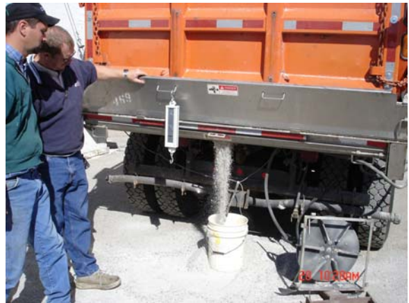
Figure 4-11 Plastic 5-gallon bucket used for catching small amounts of discharged solid material.
